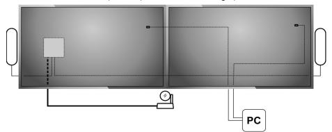
iv. Connect the USB type A/type B cable between the Display Hub and the meeting computer.
