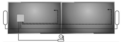
iv. Connect the CAT6 cable from the Table Hub to the Display Hub.
