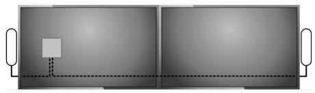
ii. Connect the USB C cable between the camera and Display Hub. The camera draws more power than normally available from an USB port and so must be connected to the Display Hub. Note, the camera can optionally be mounted upside down and an internal sensor will automatically invert the image and remote control function.
