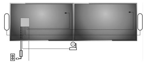
vi. NOTE REGARDING HDMI SIGNALS: Up to one 4K 60fps (YCbCr 4:2:0) on HDMI 1 or two 1080p signals (one at 1080p 60fps and one at 1080p 30fps, which is then upscaled to 60fps) can be carried between the Table Hub and Display Hub. The HDMI signals are a straight pass through between the hubs.
