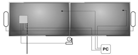
v. Connect the CAT6 cable between the Display Hub and the Table Hub.
