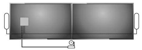
iii. Connect the HDMI cable(s) between the display(s) and Display Hub. If using just one display, connect it to the HDMI 1 jack on the Display Hub.
