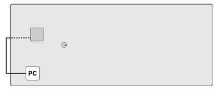
ii. Connect the HDMI cable(s) between the Table Hub and computer. Note that Rally can pass through two HDMI signals from the computer to drive two displays. If using just one display, connect it to the HDMI 1 jack on the Table Hub.
