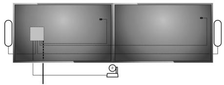
v. Connect the power supply to the Display Hub.
