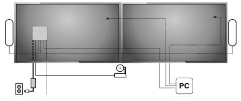
vi. Connect the power supply to the Display Hub.
