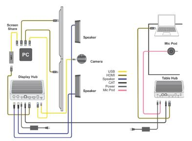
b. Using Logitech Tap with Rally, the recommended connections are as follows:
