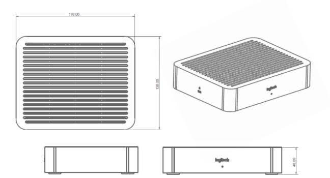
c. DISPLAY HUB: Connection point for the speakers, HDMI to the displays (when the meeting computer is connected to the Table Hub) and the meeting room computer when located at the display. Note, the HDMI signals are a straight pass through between the hubs.
