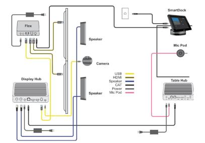
c. When using Logitech Flex with SmartDock and Rally, the recommended connection schematic is below:
