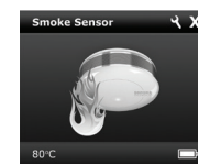
Fig. 5 Smoke Sensor icon in Fibaro Home Center indicating the fire alarm
